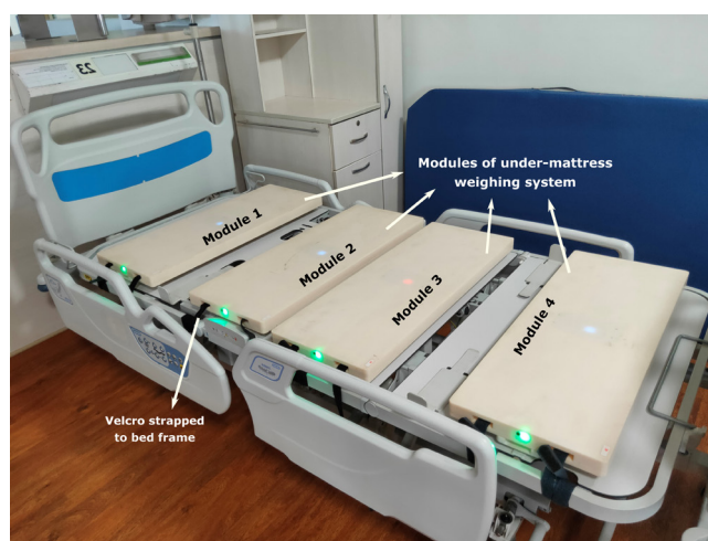
Fig. 1. Top view of the in situ under-mattress weighing device, with mattress removed. The modular devices (modules 1–4) are placed on top of 4 panels of the hospital bed frame. Velcro straps fasten the devices to the side of the bed frame. For a 4-panel hospital bed, 4 modules make up the weighing device.
