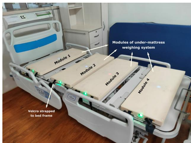
Fig. 1. Top view of the in situ under-mattress weighing device, with mattress removed. The modular devices (modules 1–4) are placed on top of 4 panels of the hospital bed frame. Velcro straps fasten the devices to the side of the bed frame. For a 4-panel hospital bed, 4 modules make up the weighing device.
