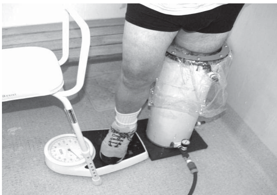
Fig. 3. Trans-tibial amputee in a normal standing posture unaided; supported by the pressure cast system.
