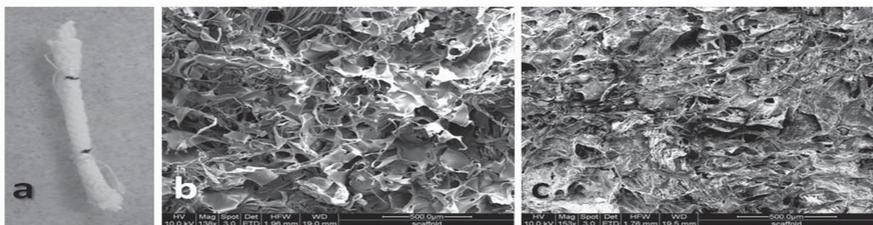
Fig. 1. (a) A rolled up triphasic silk scaffold, and (b) the SEM ultrastructure of its central sponge-coated ligament region and (c) sponge + HA-coated bone regions.
