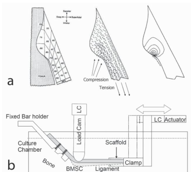
Fig. 4. (a) Physiological load distribution at the enthesis and (b) a bioreactor design for providing simultaneous compression and tension for enthesis tissue engineering.<sup>41,42</sup>
