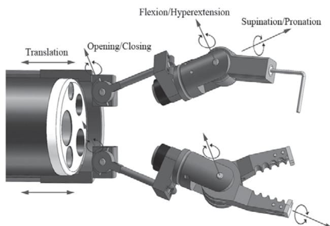
Fig. 2. Configuration of degrees-of-freedom for the robot.
