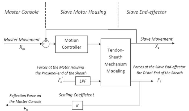
Fig. 3. Block diagram of the control architecture.
