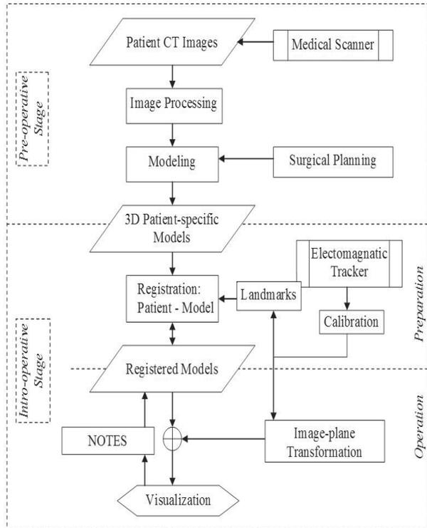
Fig. 4. Work flow of interventional navigation system.
