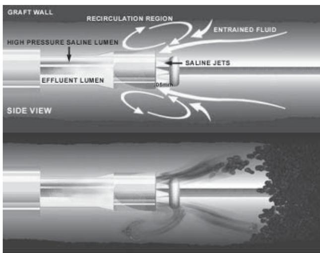
Fig. 3. The AngioJet catheter and its mechanism of action.
