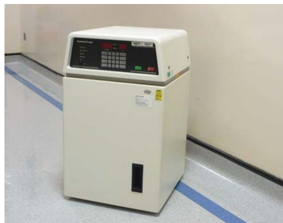
Fig. 4. A portable piece of X-ray equipment, the faxitron, which can carry out specimen radiographs within the pathology laboratory.
