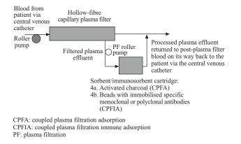
Fig. 4. Diagrammatic representation of (a) coupled plasma filtration adsorption (CPFA), and (b) coupled plasma filtration immunoadsorption (CPFIA) extracorporeal blood circuits.
